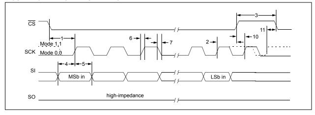
FIGURE 2-6: SPI OUTPUT TIMING
