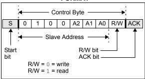
FIGURE 1-3: SPI CONTROL BYTE FORMAT
