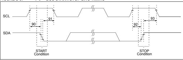
FIGURE 2-4: I<sup>2</sup>C™ BUS DATA TIMING
