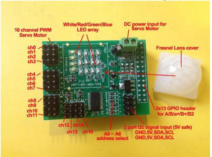
This PWM RGB-W LED HAT Board can control 16 servo motors and 16 RGB-W LEDs. The i2c PWM 16 channels can be used by all Raspberry Pi models.
