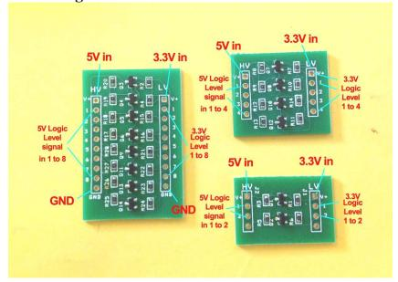
The logic level converter Set is a small PCB which safely allows you to interface devices which steps down 5V signals to 3.3V signals and step up 3.3V signals to 5V.
