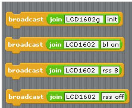
command "LCD1602g init" initial GPIO 16x2 LCD
