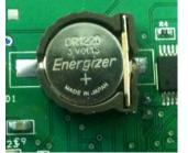
First Install battery for RTC , " + " mark on top RTC DS1307 - 68 in i2cdetect –y 0 or i2cdetect –y 1 for Rs-Pi V2 you will see 68 in the screen 68 -> RTC DS1307 48 -> tmp102
